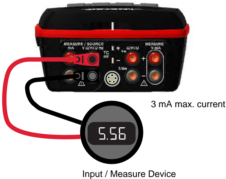
Figure 18 Connections for Testing an Output Device
