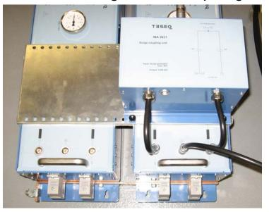
■ IEC Line to line coupling trough 18µF
