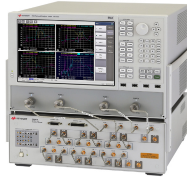
Figure 14. Multiport configuration with E5080A and E5092A
