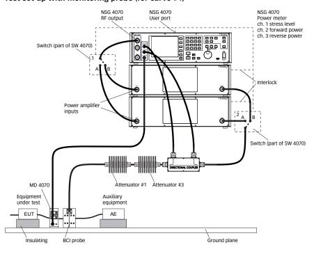
Attenuator #1: 10 dB, 30 W Attenuator #2: not in use Attenuator #3: not in use Termination: 50  $\Omega$  10 W
