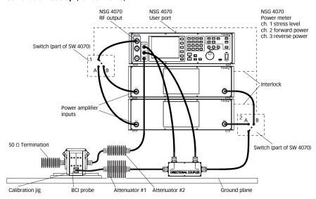
Attenuator #1: 10 dB, 30 W Attenuator #2: not in use Attenuator #3: not in use Termination: 50  $\Omega$  10 W
