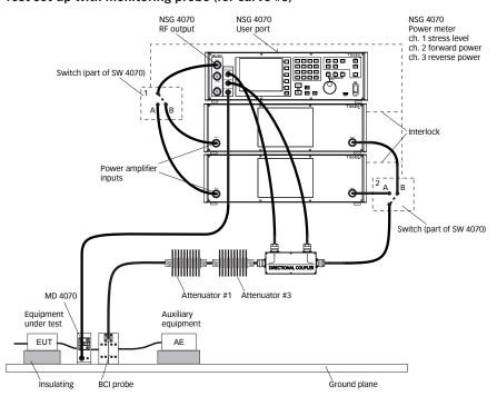
Attenuator #1: 10 dB, 30 W Attenuator #2: not in use Attenuator #3: 10 dB, 30 W Termination: 50  $\Omega$  10 W
