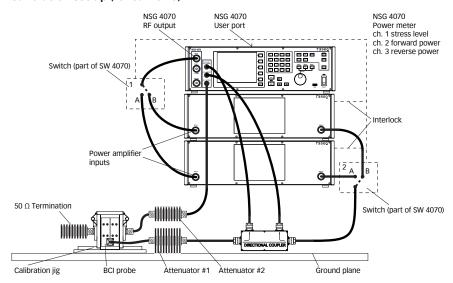
Attenuator #1: not in use Attenuator #2: 10 dB, 30 W Attenuator #3: not in use Termination: 50  $\Omega$  10 W
