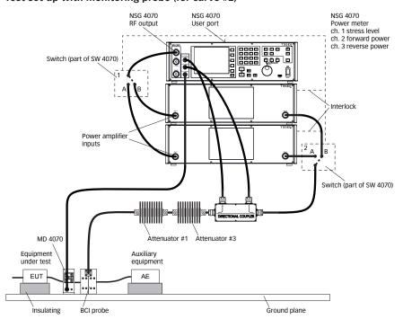
Attenuator #1: 10 dB, 30 W Attenuator #2: not in use Attenuator #3: 16 dB, 30 W Termination: 50  $\Omega$  10 W
