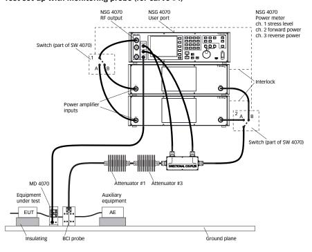
Attenuator #1: 10 dB, 30 W Attenuator #2: not in use Attenuator #3: 20 dB, 30 W Termination: 50  $\Omega$  10 W
