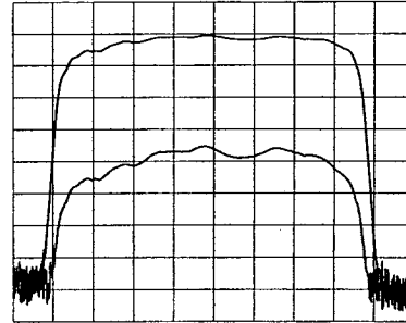
Figure 4.4 Swept third-order distortion measurement of an IF amplifier and filter. Distortion level is the difference between the reference trace (upper) and the measurement trace (lower). Vertical axis 10 dB/div.; Horizontal axis 429 kHz to 479 kHz.
