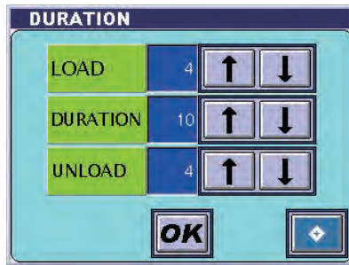
In addition to the test force dwell time, you can specify loading and unloading testing actions.
