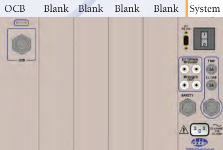
Figure 2. Minimum Configuration for Circuit Breakers
