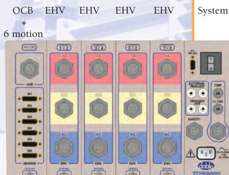
Figure 4. Circuit Breaker Configuration with 6 Motion Channels
