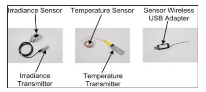
1. Before starting the PVA software, connect the Sensor Wireless USB Adapter to a USB port in your computer.
