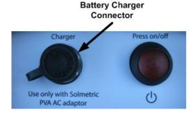
Charging the battery can take up to 6 hours. Once the battery has been charged, the PVA-600 will operate for approximately 2 days of normal use. During heavy use, nightly charging is suggested.
