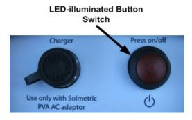
Press the power button once on the I-V Measurement Unit.
