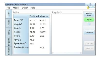
Press the **Snapshot** button to temporarily store measured values for comparison with subsequent measurements. Temperature and irradiance values appear in the Predicted column if they are being derived from the measured I-V curve.
