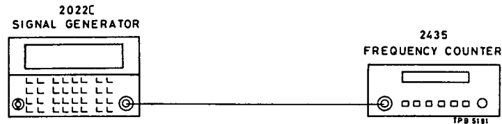
Fig. 5-2 Test gear arrangement to check frequency accuracy
