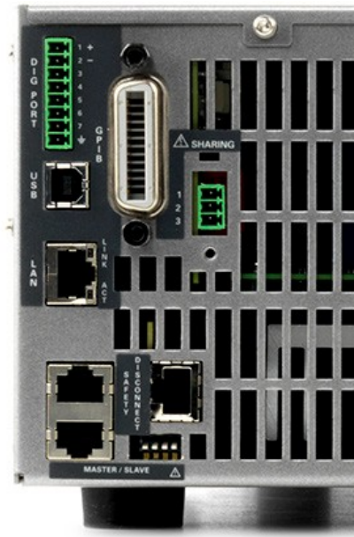
Figure 6. Digital control port on rear panel
