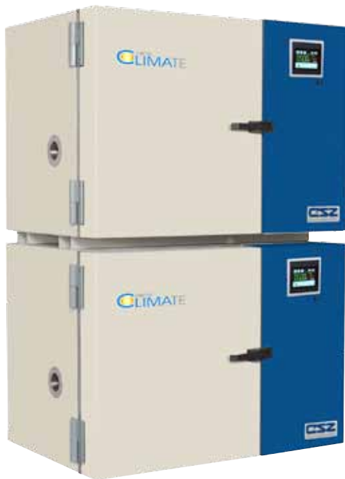
MicroClimate Benchtop Temperature Chamber shown in the stacked position.
