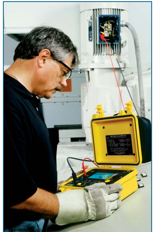
Large display and buttons make the Model 1060 ideal for shop use even with gloves.
