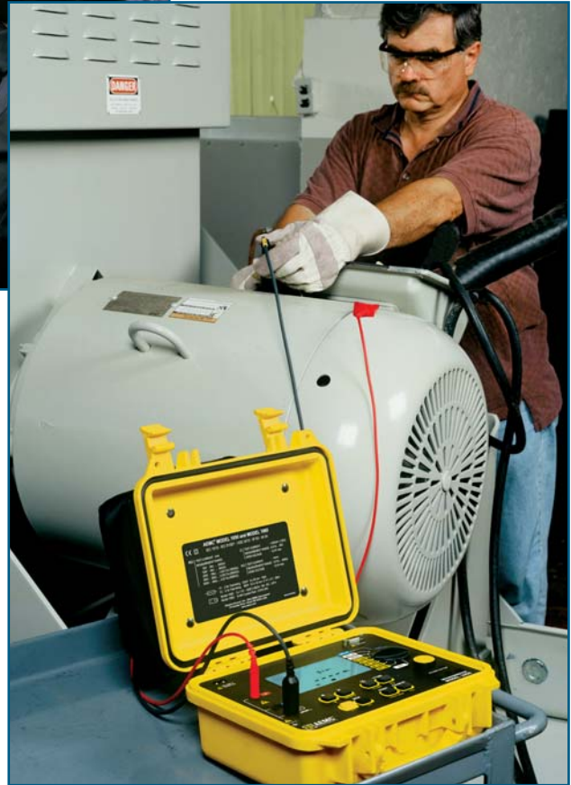
Model 1060 checking insulation resistance between windings on a three-phase motor.
