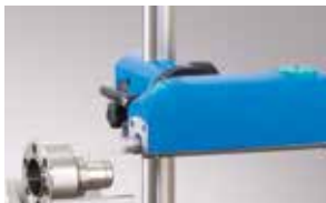
Motorized lowering of the probe
