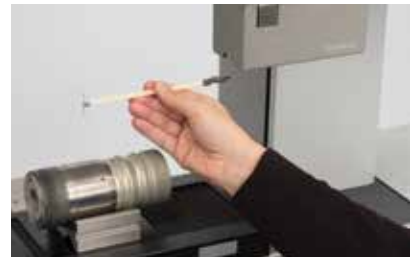
Probe arms with magnetic coupling
