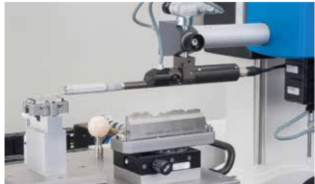
Automated calibration of the measuring system via integrated standards
