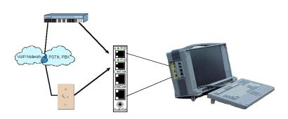
Step 5. Start the VQT software on the controlling PC or VQT Portable Analyzer (see page 60).
