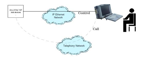
With the client license key enabled, the VQT Portable Analyzer can control other VQT devices in a VQT test system.
