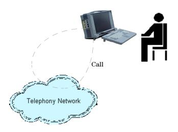
The VQT Portable Analyzer can act as both end points of the call for most interfaces. When using the 10/100 Ethernet interface, you need a VQT device at both ends of the call.
