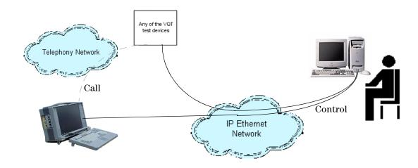
The controlling device can manage multiple VQT servers across an IP network. Those VQT servers can run voice quality tests and the measurement results will be sent to the controlling PC for display.
