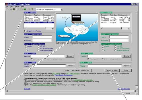
If you plan to perform locally controlled, single-server testing, click Local in the Server Lists, select the acquisition hardware, click the Start Client/Server Connections button, and begin testing.
