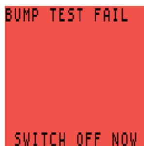
Figure 48: Bump Test Fail - Switch Monitor OFF
