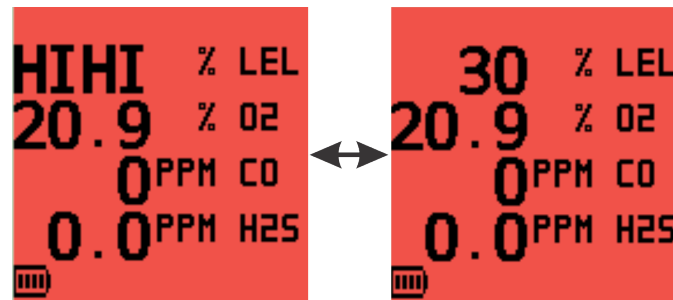
Figure 26: LEL HIHI Alarm
