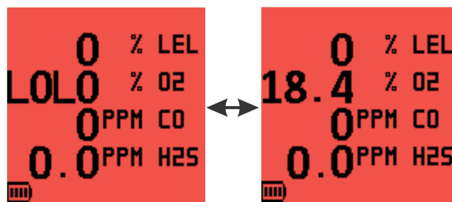
Figure 25: O 2 LOLO Alarm
