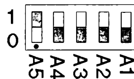
Figure 4-15. HP-IB Address Switch (Factory setting)
