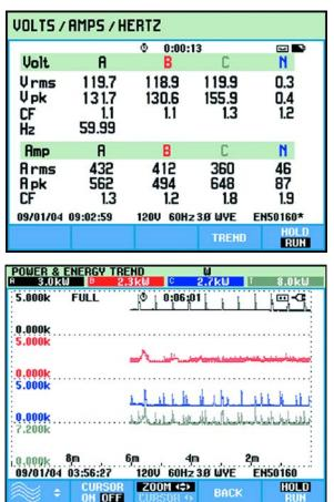
AutoTrend automatically records all displayed parameters in the background. Toggle between data and trend view and use cursors and zoom to analyze measurements without interrupting the recording.
