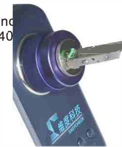
LC transceiver Inspection
