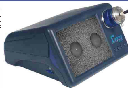
MPO Connector Inspection
