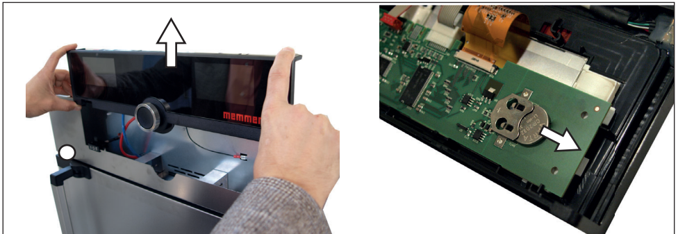
Fig. 34 Removing the lithium battery
