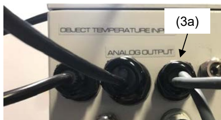
Figure 29: Connection cable on the "Object temperature input" connection (3a)
