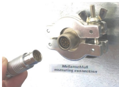
Figure 28: Measuring connection (12) with measuring access port
