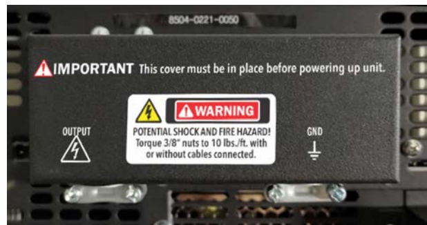
Figure 3.3 – Output Safety Cover
