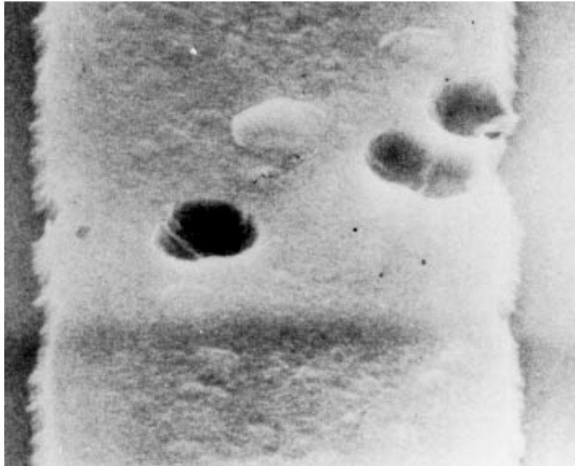
FIGURE 2077-20. General metallization voids at 5,000X (reject).
