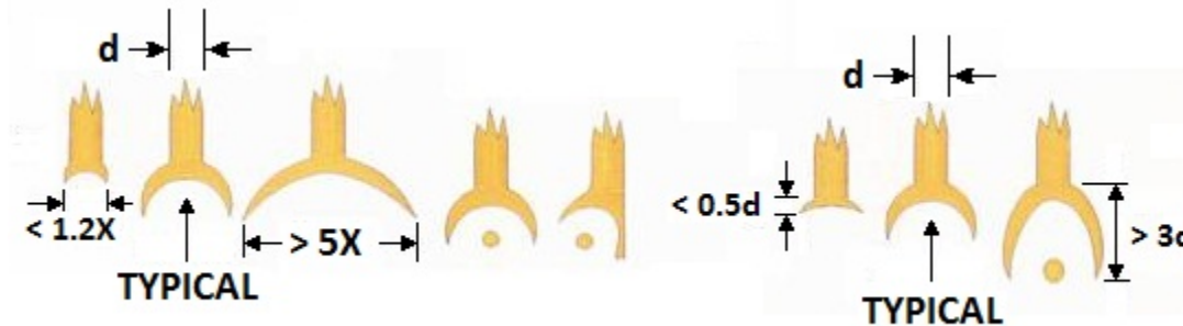
FIGURE 2072-23. Tailless bond dimensions.
