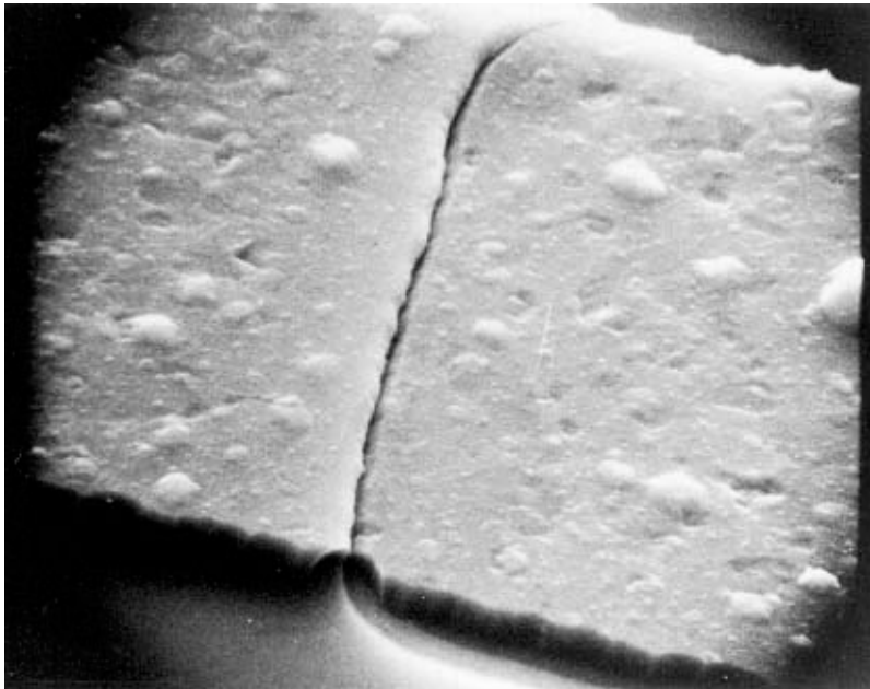
FIGURE 2077-9. Tunnel/cave at oxide step at 5,000X (reject).
