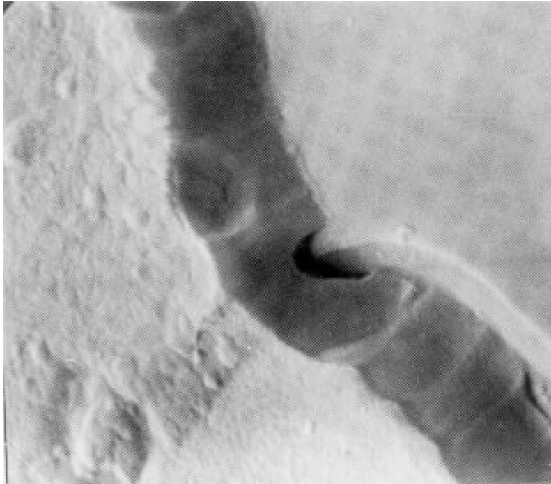
FIGURE 2077-8. Tunnel/cave at oxide step at 10,000X (accept).
