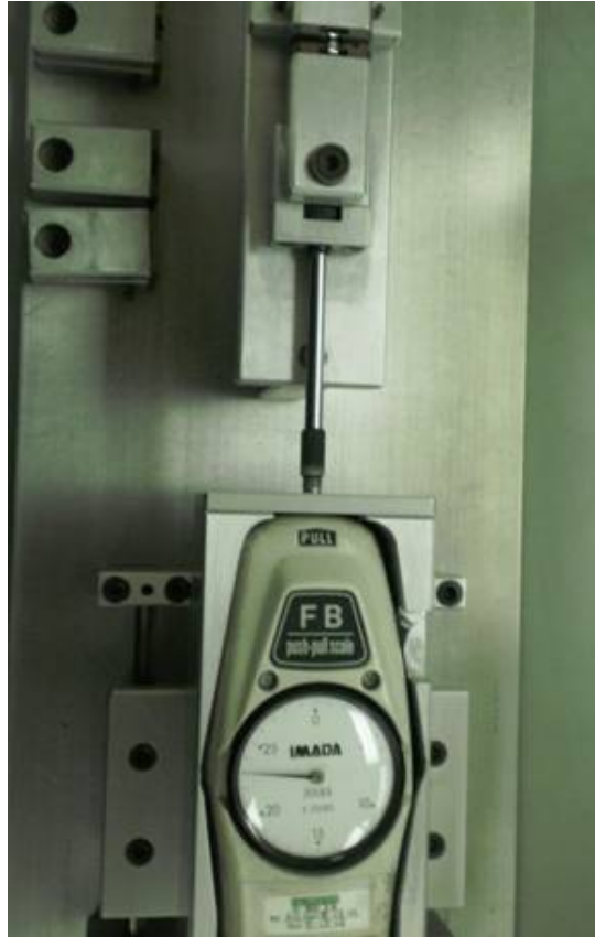
FIGURE 2038-1. Sample apparatus fixture with force measuring gauge.
