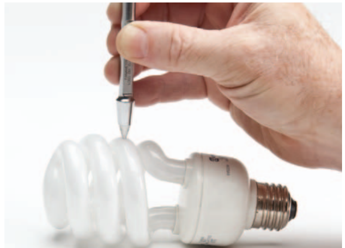
The High Resolution software option allows thickness measurements of up to 0.001 mm (0.0001 in.) resolution.
