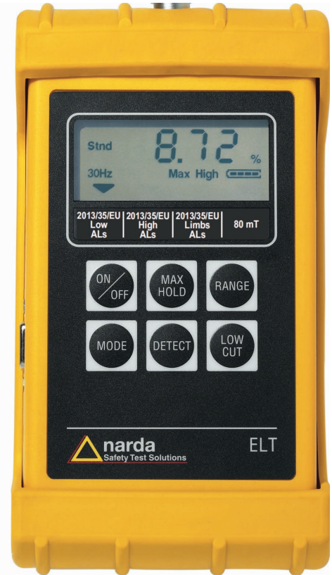
In Exposure STD mode the result is displayed directly as a percentage of the permitted limit
