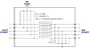
The frequency range of the test is from 150 kHz up to either 80 or 230 MHz. The test level is typically 1, 3 or 10 Vrms with the test signal 80%, AM modulated with a 1 kHz tone. A typical test setup is illustrated below.
