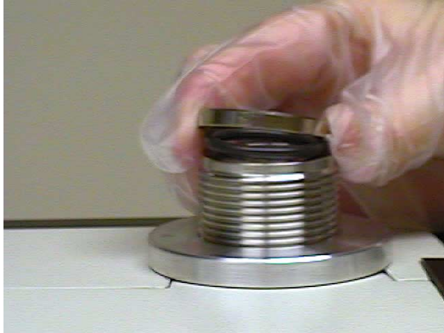
Figure 4-14 Remove the Test Port Compression Ring and O-ring
