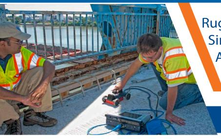
Rugged, High-Performance Single-Channel GPR Data Acquisition System
