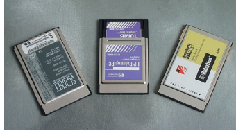
N1618A: 56K/v.90 Modem PC Card N1620A: 10BaseT Ethernet LAN PC Card N1621A: Compact Flash and PCMCIA Adapter
