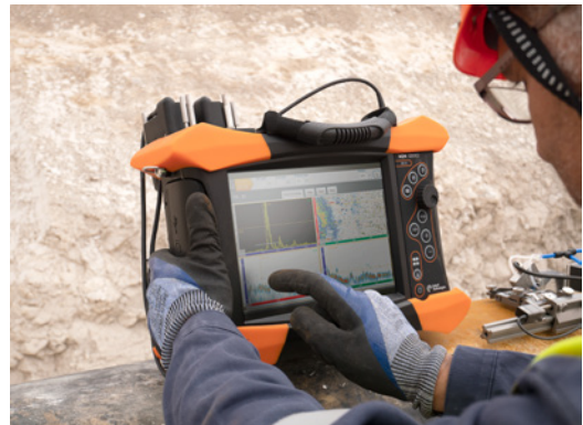
In-field inspection using M2M Gekko
