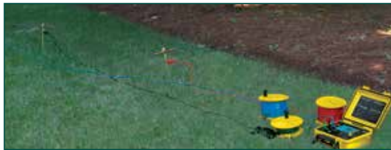
The Model 6472 provides an automated way to measure the value of the earth/ground using the Fall-of-Potential method and storing measurements.
