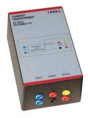
IEC/EN 61000-4-19 specifies the differential current test in the frequency range 2 kHz to 150 kHz. Teseq offers with CT 419-5 a transformer with integrated matching network for testing EUTs like electricity meters. The CT 419-5 is fully compliant with the requirements of the standard and provides a simple and reliable method of injecting differential mode current into the equipment under test (EUT).
