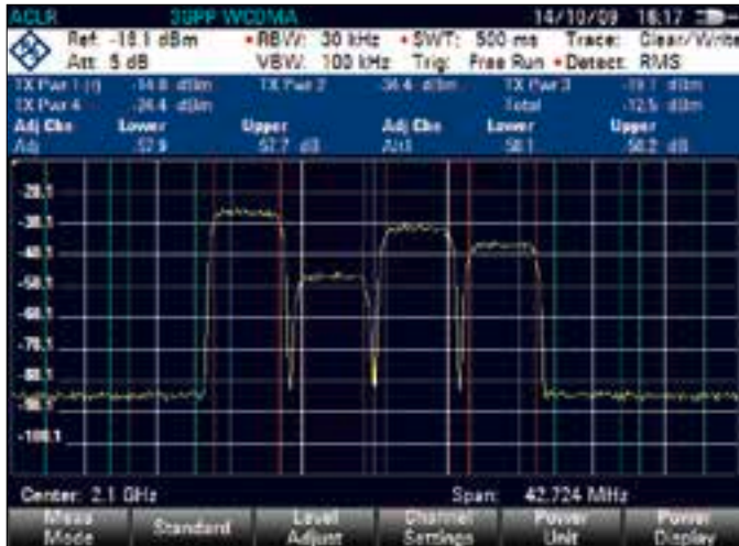
ACLR measurement on a 3GPP WCDMA signal with four carriers.
