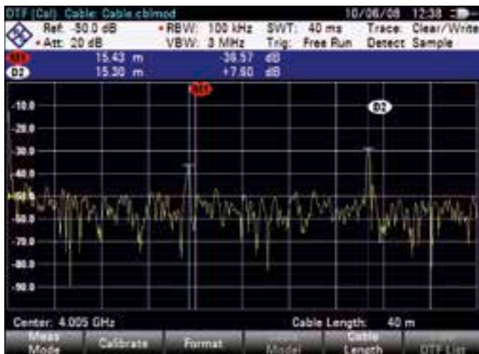
Distance-to-fault measurements (DTF).
