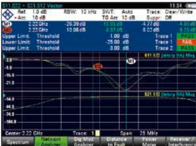
Vector network analysis: simultaneous display of four S-parameters.
