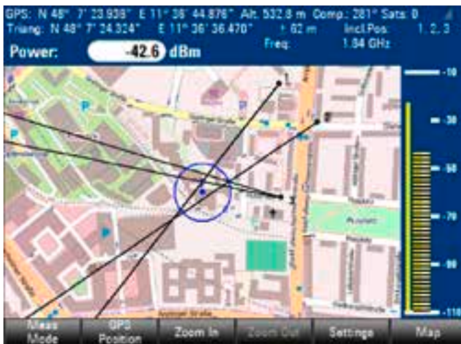
Display of map triangulation lines with R&S®FSH-K15
