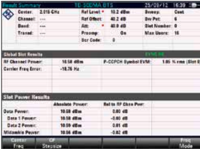
Analysis of TD-SCDMA transmit signals.
