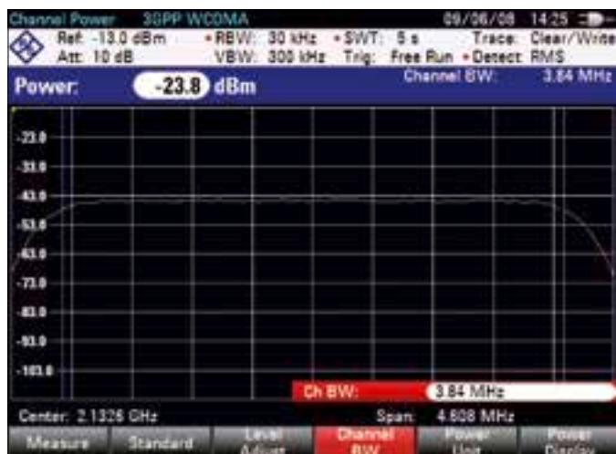
Channel power measurement.
