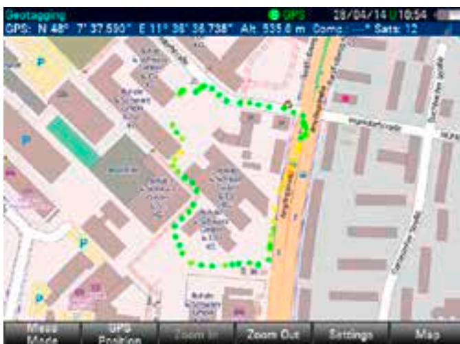
Geotagging results display with R&S®FSH-K16
