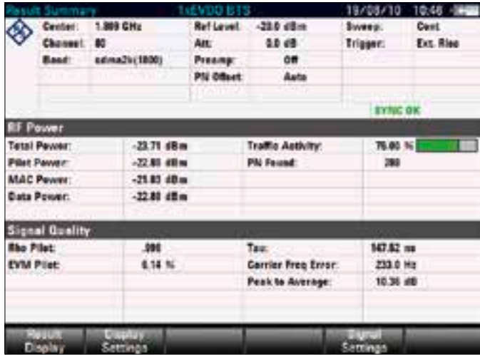
Analysis of a 1xEV-DO transmit signal with the R&S®FSH-K47 option.
