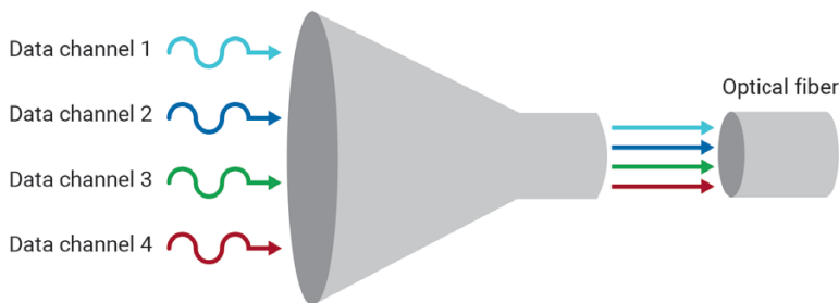
Figure 1. WDM acts as an “optical funnel” using different colors of light (wavelengths) for each signal.
