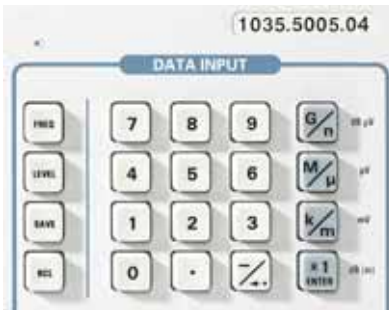
FIG 9: SAVE and RCL for storing and recalling settings
