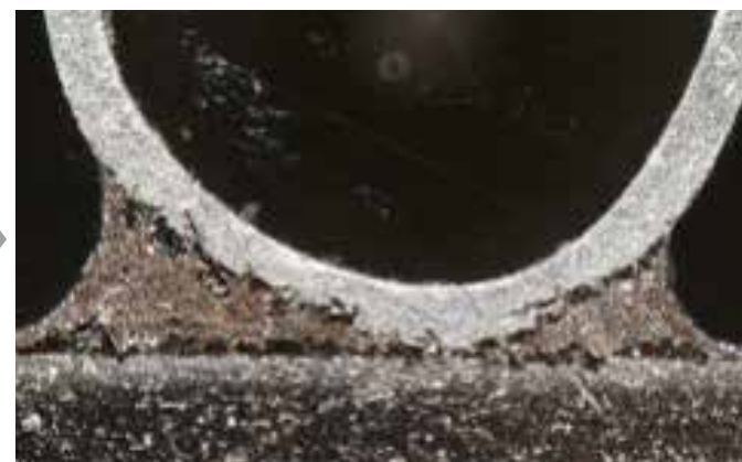
DSX1000 Polized observation (300X), clearly visualize the peeling of the weld
