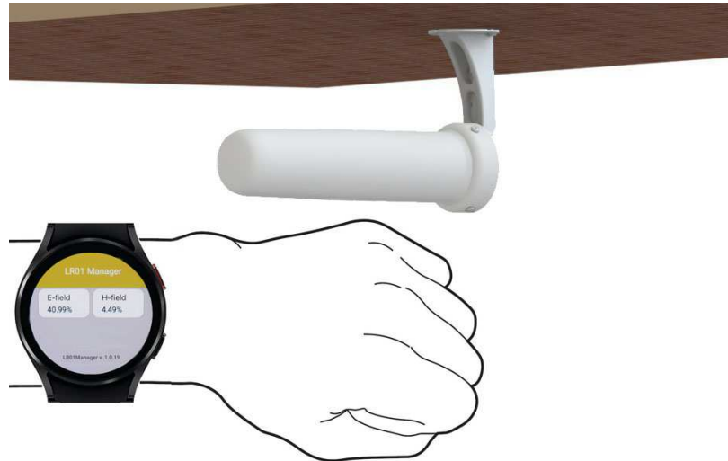
Fig. 2-7 AMC link with Bluetooth communication by smartwatch
