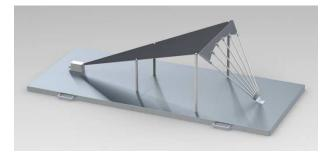
This test set-up can be used for the susceptibility testing of small pieces of equipment such as printed boards, small subsystems, etc., according to MIL-STD-461 / RS105 (NEMP: nuclear electromagnetic pulse). Associated with the generator EMP25K-2-23, the minimum field under the line RL50-50 is 50 kV/m at full output. Even higher fields can be achieved for smaller objects placed close to the beginning of the line. The line can also be used for other pulse or CW tests.
