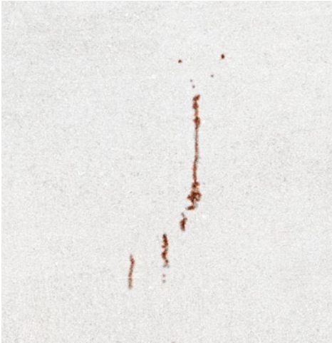
Part inspected with Penetrant Testing (visible red dye)
