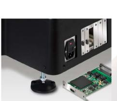
**CANBUS Interface** provides fast, accurate communication between the LD Series and add-on accessories like extensometers and temperature chambers.
