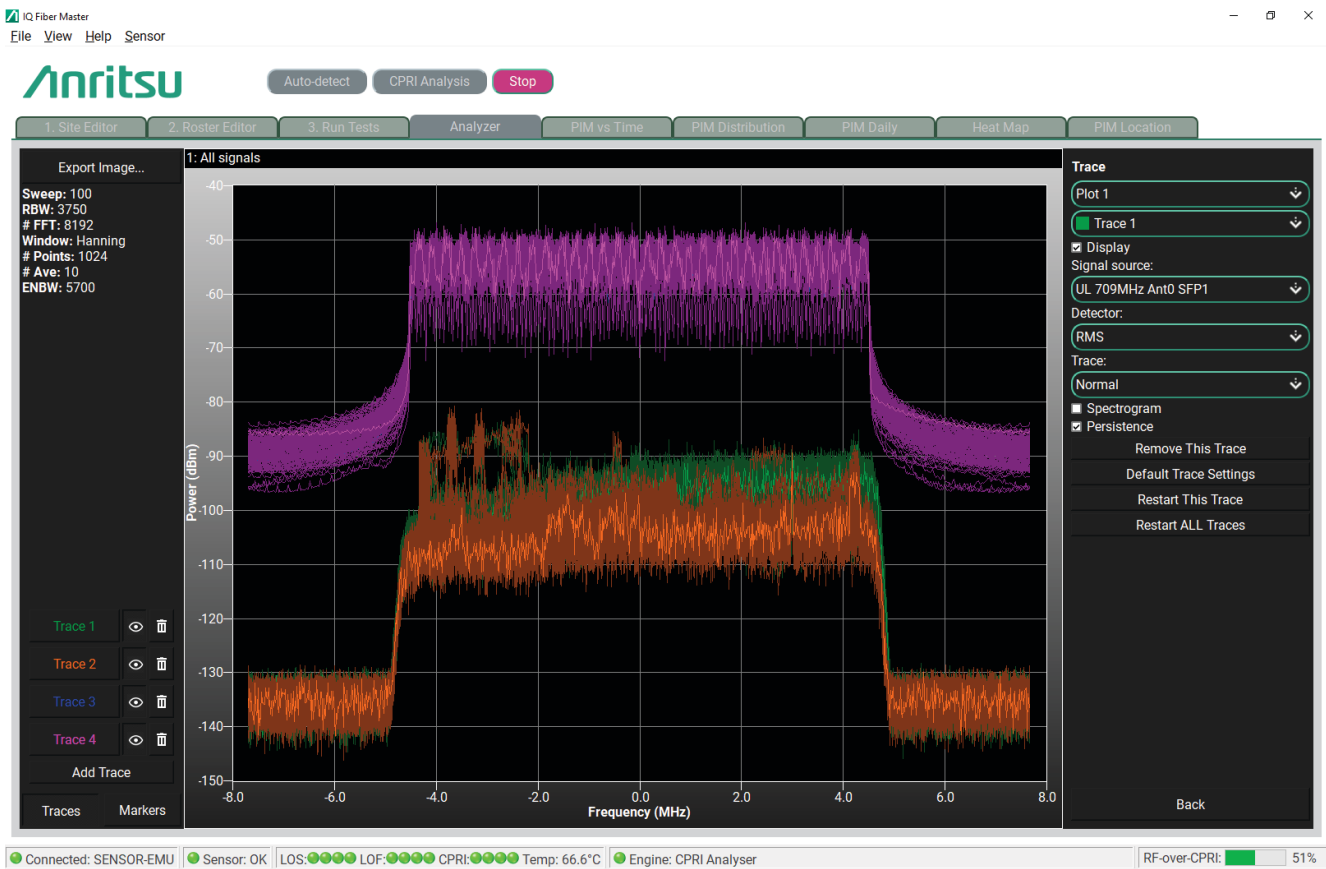
Figure A-10. LTE RF over CPRI display
