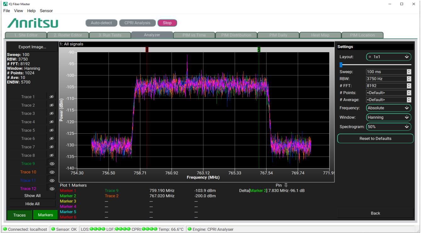
Figure 3-8. Analyzer tab: Standard Relative Spectrum View (dark) with Markers and Side bars
