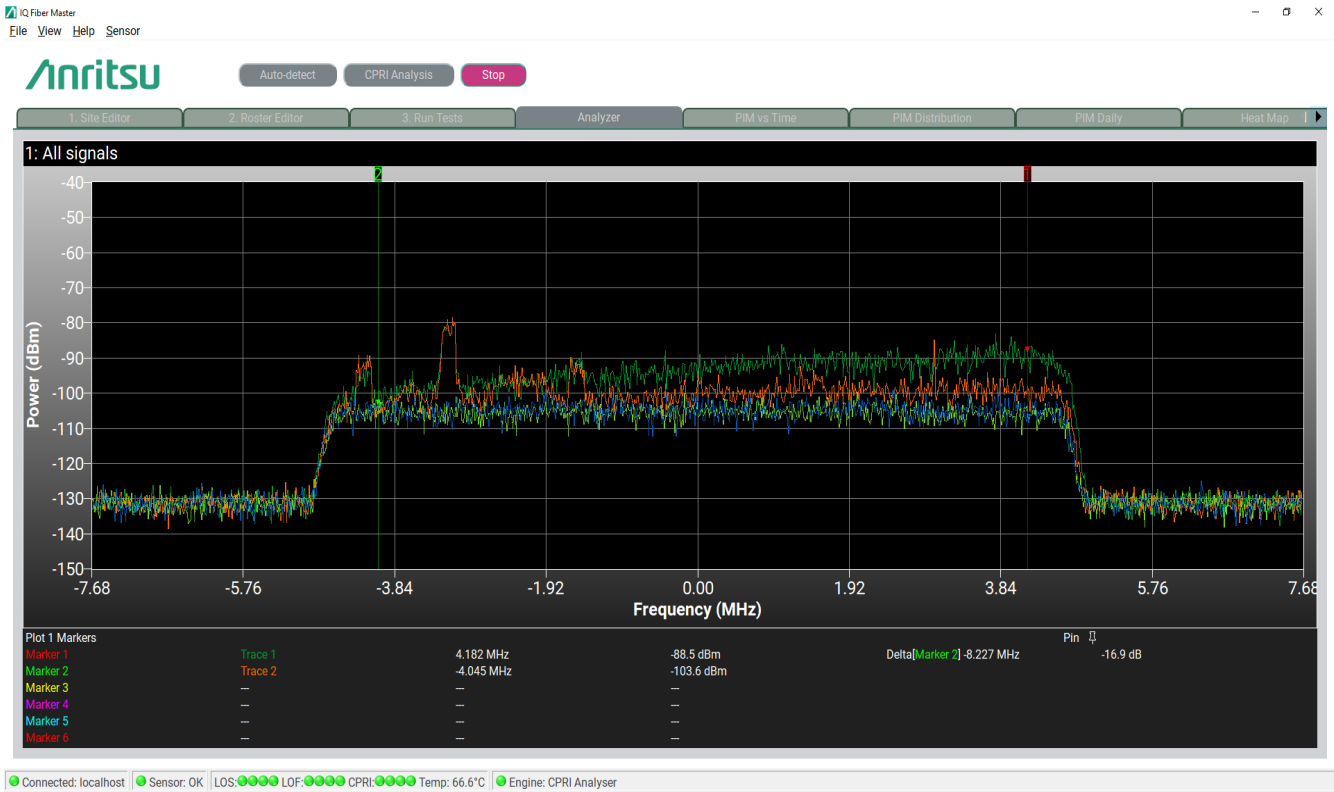
Figure 3-14. Analyzer tab: Standard Relative Spectrum View (dark) with Markers and no sidebars
