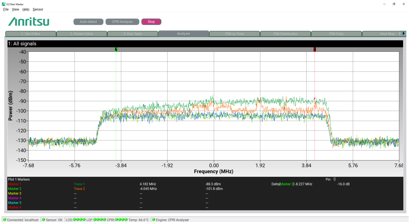
Figure 3-24. Analyzer tab: Standard Relative Spectrum View (light) with markers and no sidebars
