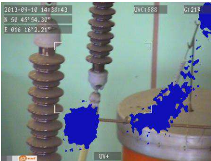
Fig. 3, 4. Corona discharge in laboratory conditions.
