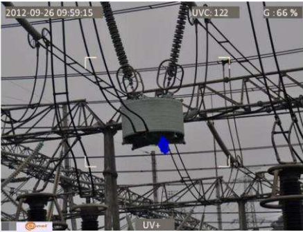
Fig. 5-8. Corona discharge in real power grids.
