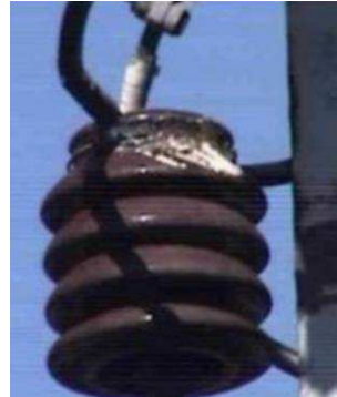
Fig. 9, 10. Corona discharge and its effects.
