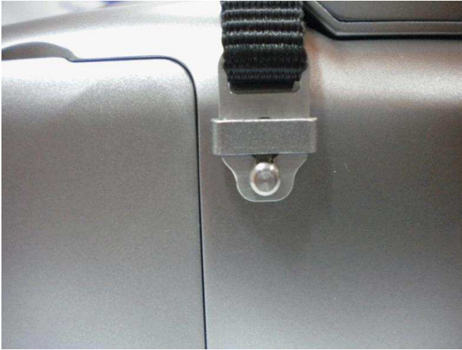
Fig. 13. Fixing strap to the holders.
