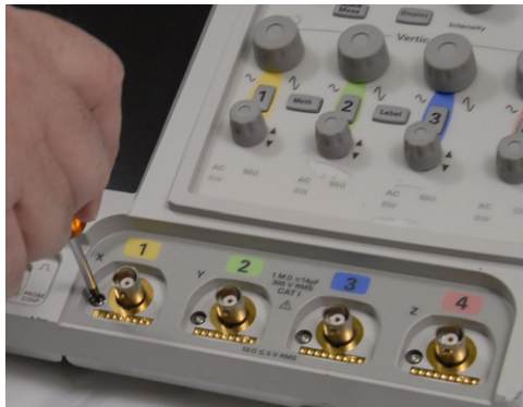
Figure 21 Removing the T6 screws
