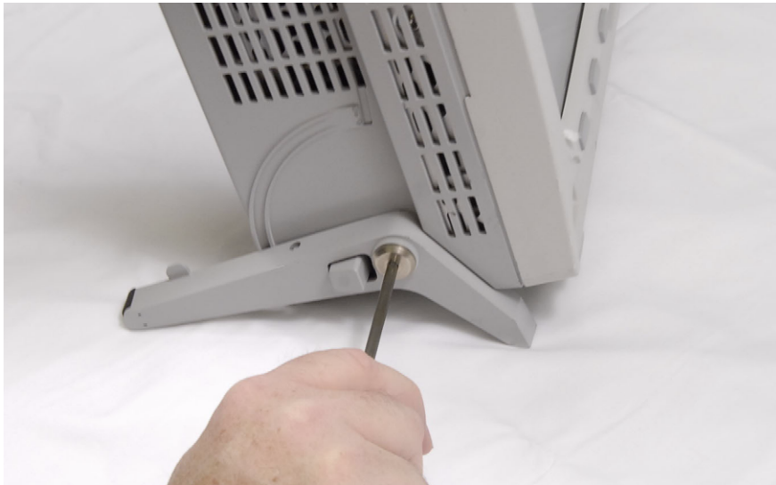
Figure 17 Removing adjustable leg
