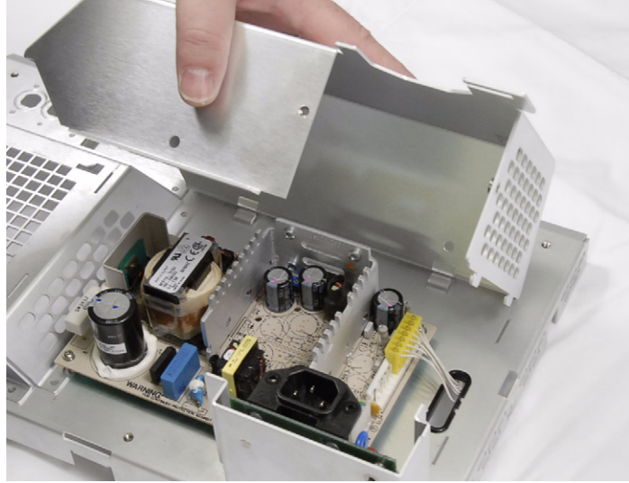
Figure 37 Lifting power supply cover off
