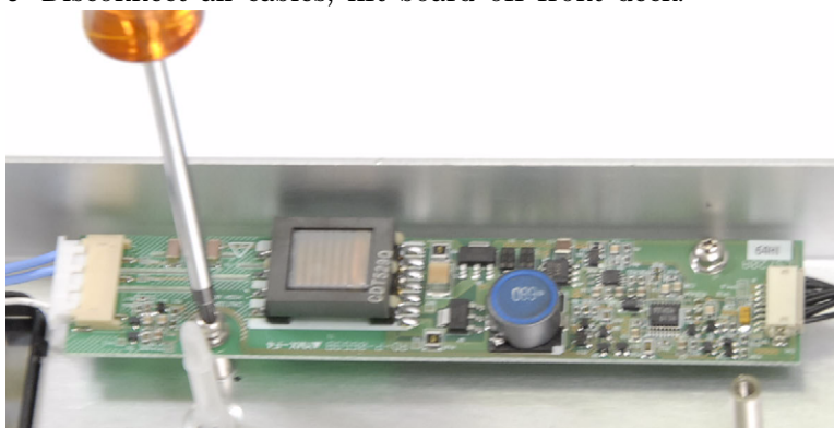
Figure 24 Removal of inverter board
