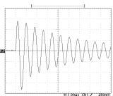
Accurate Impulses - The PIM 150 wave shape and amplitude are guaranteed to conform to specification at the CDN output. Also with simultaneous, multiple coupling path selections.
