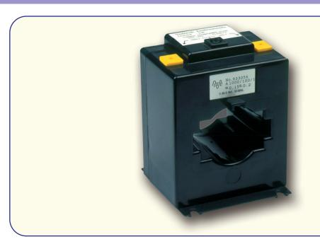
The Voltech CT1000 is a toroidally wound AC current transformer that extends the range of Voltech power analyzers such as the PM100, PM300 or PM3000A to 1200A rms. Close- tolerance current ratios provide a measurement accuracy of better than 0.2%, making the CT1000 suitable for precision-grade measurements.
