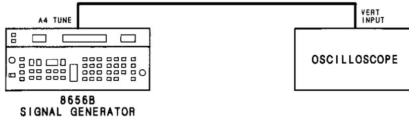
Figure 5-7. High Frequency Loop Offset Adjustment Setup
