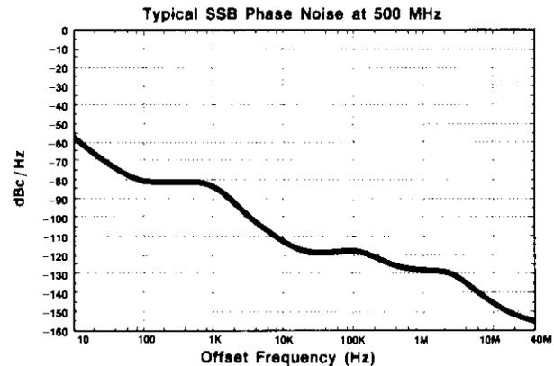
Typical SSB  $\phi$  Noise,  $f_c = 450$  MHz
