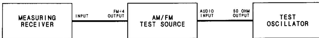
*Figure 4-9. Measuring Receiver Incidental AM Verification Test Setup*
