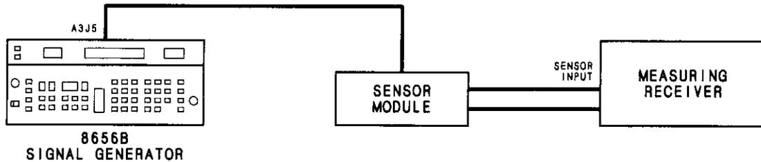
*Figure 5-10. 50 MHz Reference Oscillator Level Adjustment Setup*
