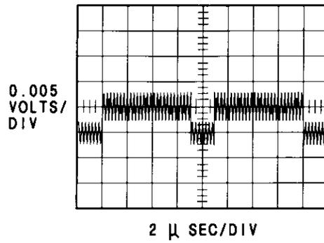
*Figure 5-21. Oscilloscope Display with Pedestal Needing Adjustment*
