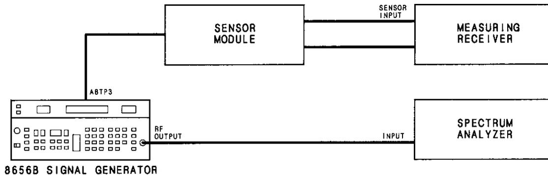
Figure 5-15. Heterodyne Band 800 MHz Bandpass Filter Adjustment Setup
