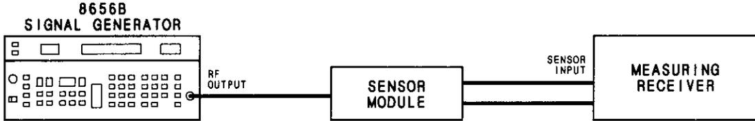
Figure 5-14. Level and ALC Loop Detector Adjustment Setup
