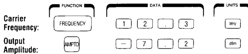
Both of the Signal Generator's carrier functions have value-selectable parameters. These parameters are selected in the Function-Data-Units format as shown in the examples above.
