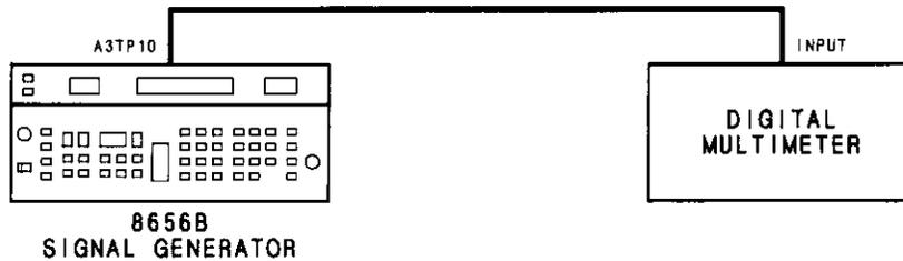
Figure 5-1. +5.4 Vdc Power Supply Adjustment Setup
