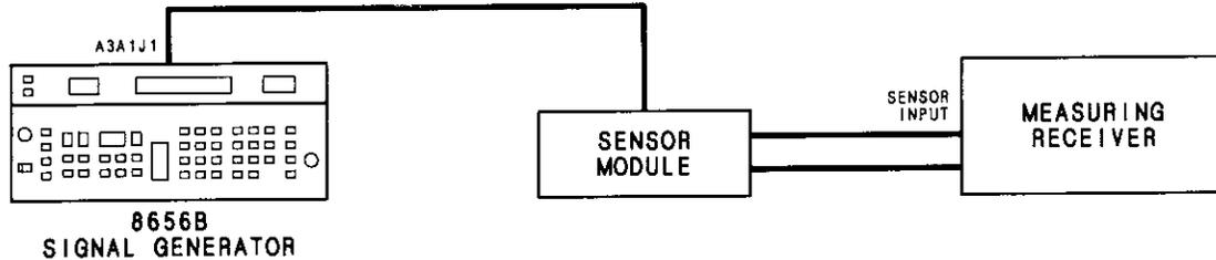
Figure 5-11. 60 to 110 MHz Oscillator Flatness Adjustment Setup
