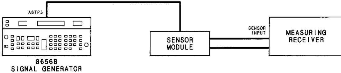
Figure 5-13. 400 MHz Bandpass Filter Adjustment Setup
