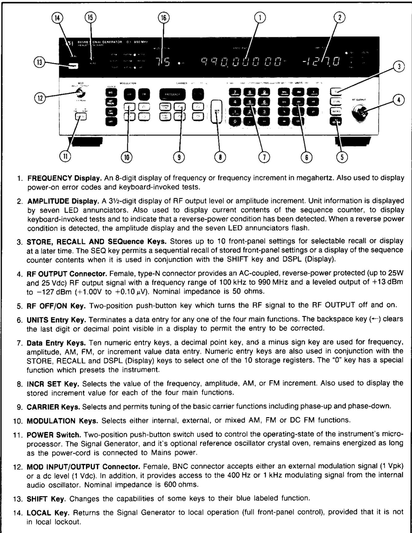
Figure 3-1. Simplified Front-Panel Features and Operation (1 of 3)
