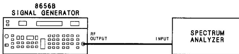
*Figure 4-1. Spurious Signals Test Setup*
