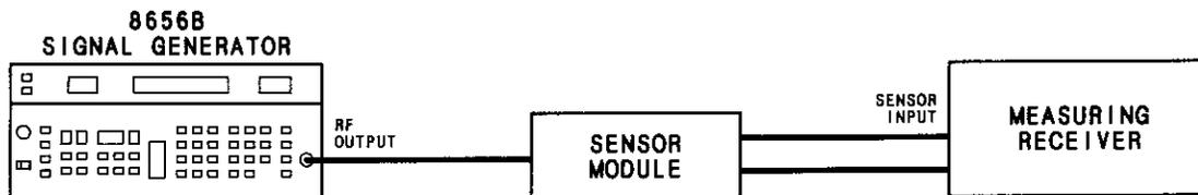
Figure 5-15A. Heterodyne Band Accuracy and Flatness Adjustment Setup
