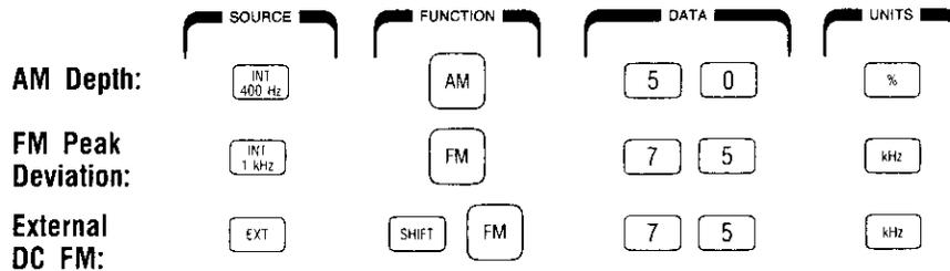
Internal, external, or mixed AM or FM functions can be selected. Modulation parameters are selected in the Source-Function-Data-Units format as shown in the examples above. One of the two internal modulation sources (400 Hz or 1 kHz) and/or a signal or dc level from an external modulation source coupled through the front-panel connector may be used to modulate the carrier.
