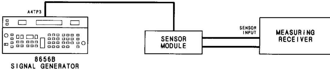
Figure 5-12. 690 to 740 MHz IF Compensation Adjustment Setup
