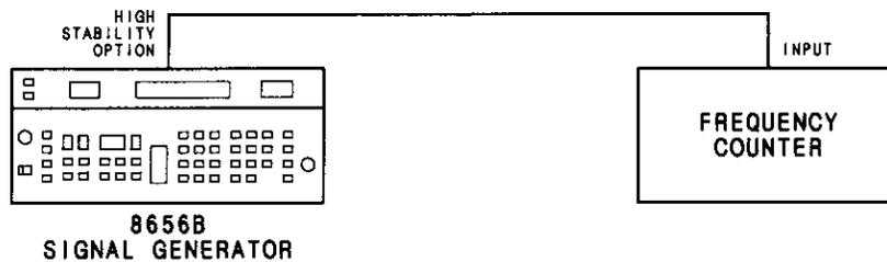
*Figure 5-26. 10 MHz Reference Oscillator Frequency Adjustment Setup*
