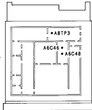
4. Zero the measuring receiver and wait for the zero LED to go out. Connect the measuring receiver to A8TP3.
