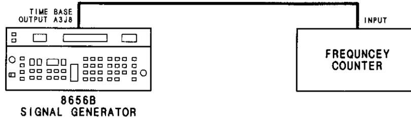
Figure 5-9. 50 MHz Reference Oscillator Frequency Adjustment Setup
