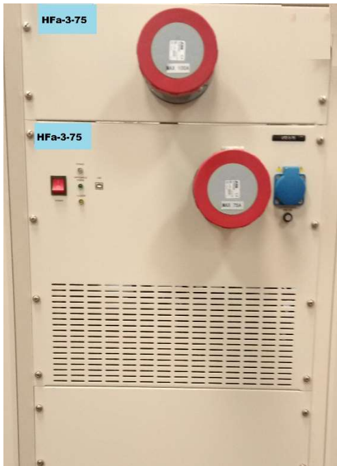
Figure 6 Part of the 19" rack, showing the HFa-3-75, and the Impedance units behind the louvered front panel.
