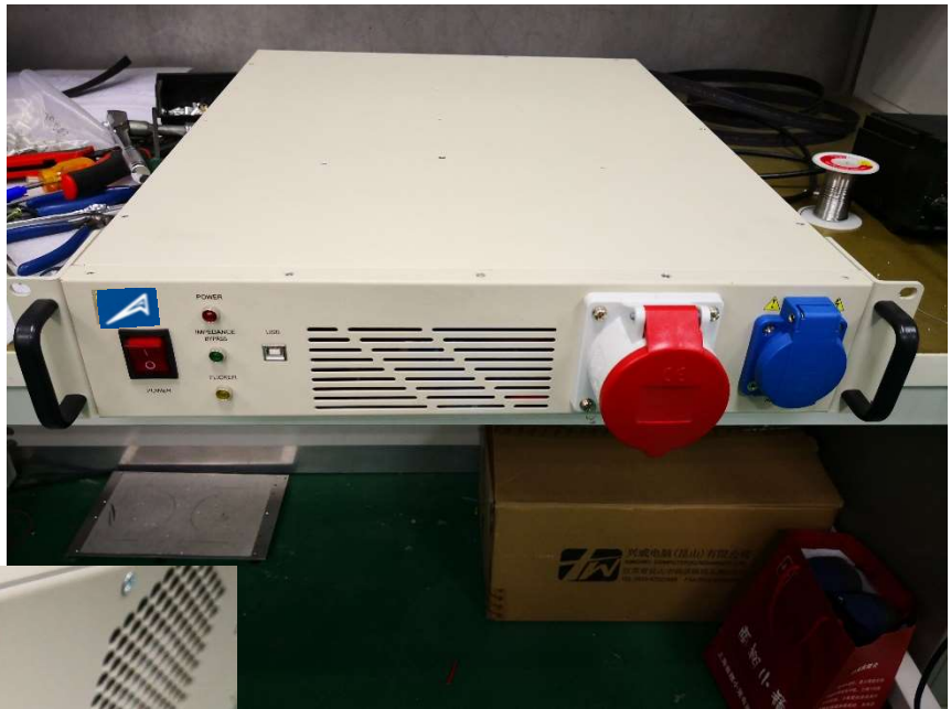
Figure 47 The HFA-3-36 – 19" form factor with built-in Reference impedance
