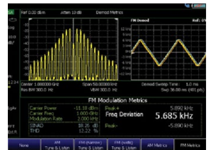
Characterize AM/FM signals using AM/FM demodulation
