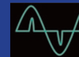
Programmable Output Impedance Same conditions as above with programmable Z_o engaged. THD=0.25%
