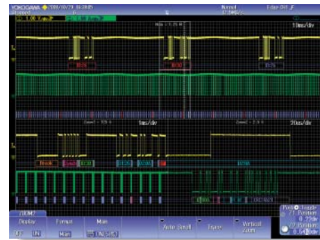
Simultaneous analyses of CAN and LIN
