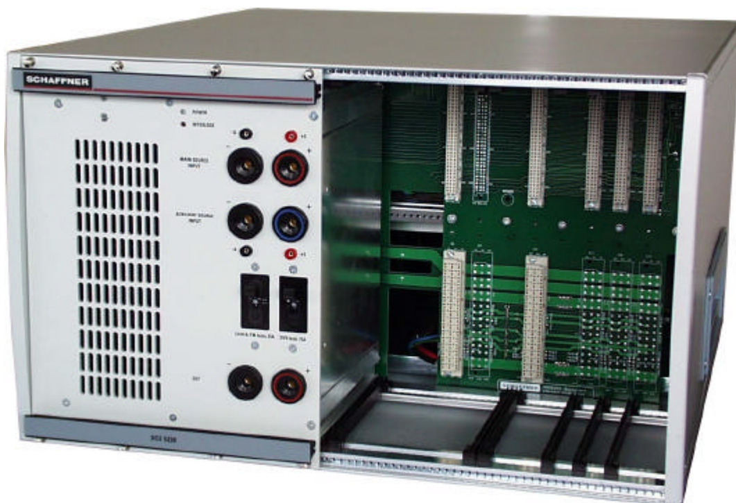
Figure 5.4 – DCS 5230 Module Installed in Left-Most Slot in Basic Chassis
