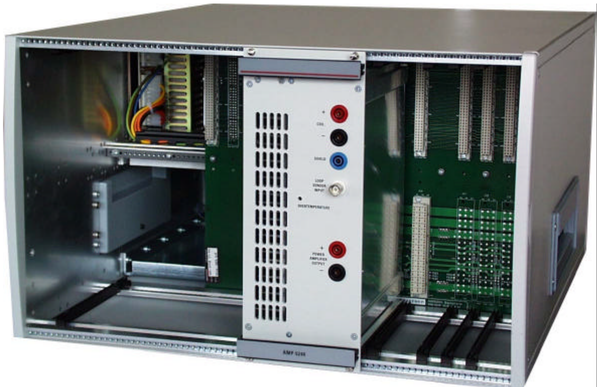
Figure 6.3 – AMP 5240 Module Installed in the Centre Slot in the Basic Chassis
