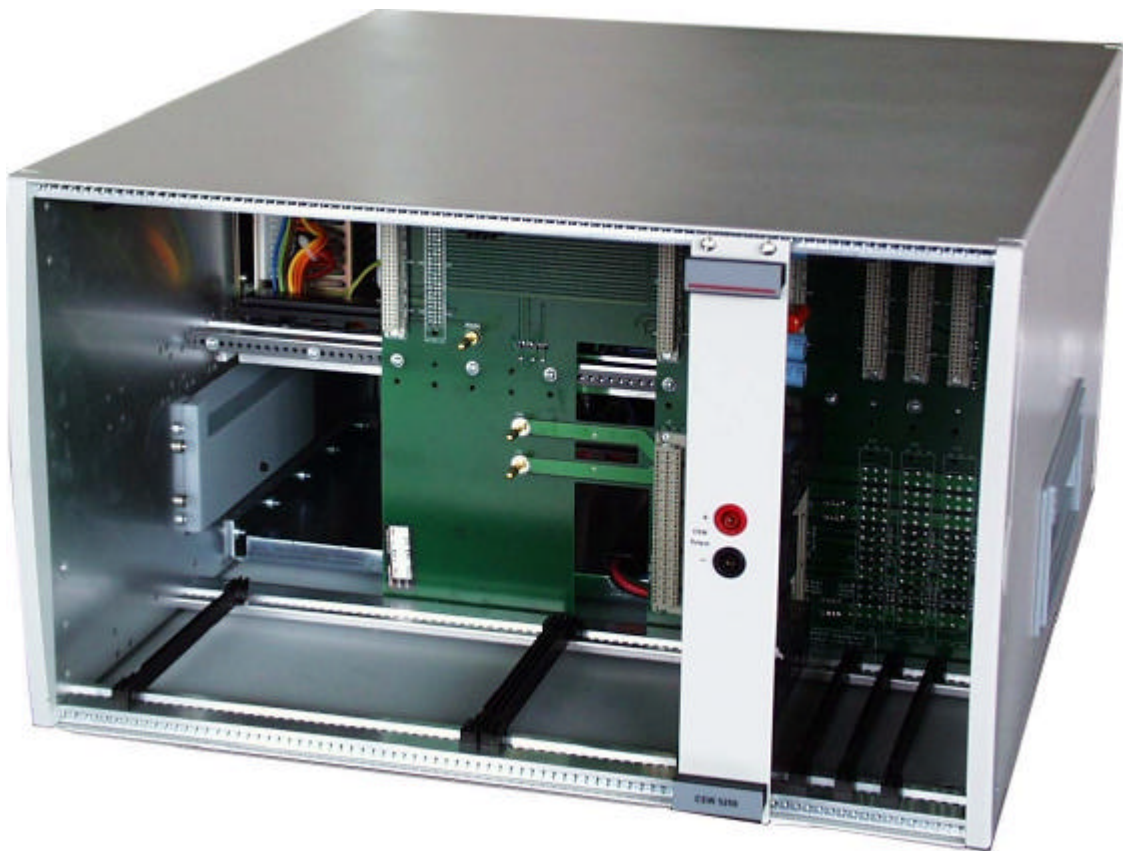
Figure 7.3 - CSW 5250 Module Installed in the Basic Chassis
